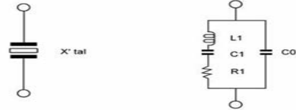
Fig 1 Equivalent Circuit of Crystal Unit
